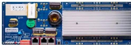
RS485 Communication between battery and inverter Band rate:9600bps RS485 Interface Communication between parallel packs of BMS and PC Band rate:9600bps
